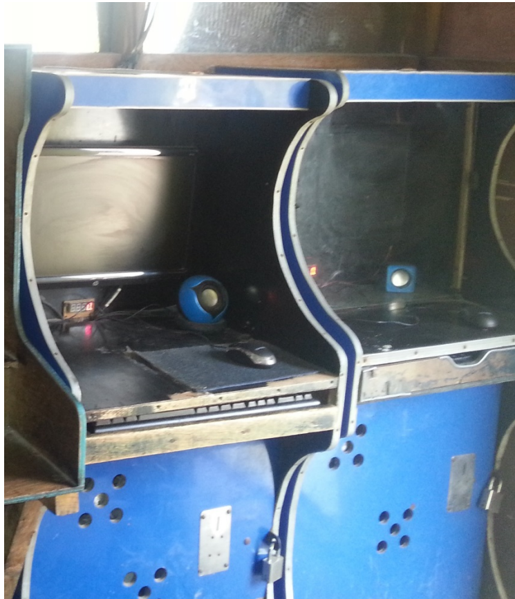
Figure 1. The pisonet. A computer in a locked wooden casing, it runs with a coin-operated mechanism and a timer.
