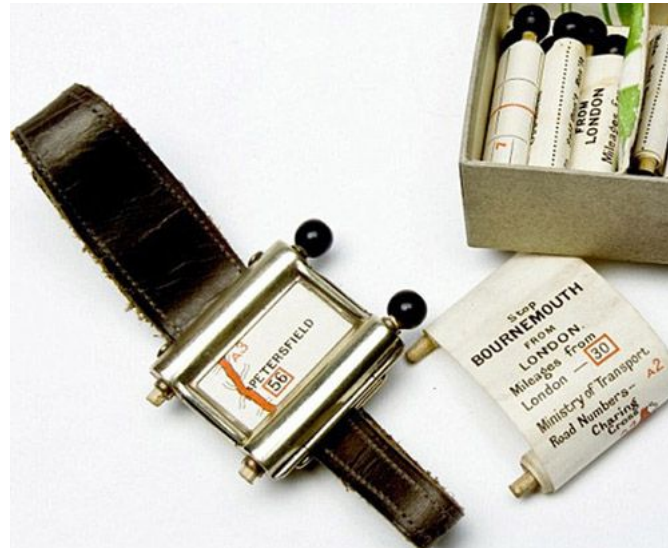
Figure 4. The Plus Four Wristlet Route Indicator, 1927, with accompanying miniature scroll maps (Chan, 2010).
