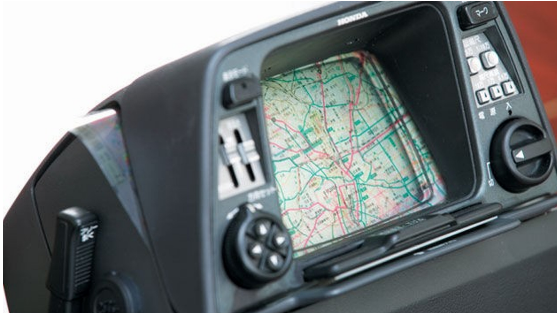
Figure 5. An early in-car navigation system: Honda's Electro Gyroator from 1981. ( https://autoweek.com/article/technology/1981-honda-invents-first-car-navigation-system ).
