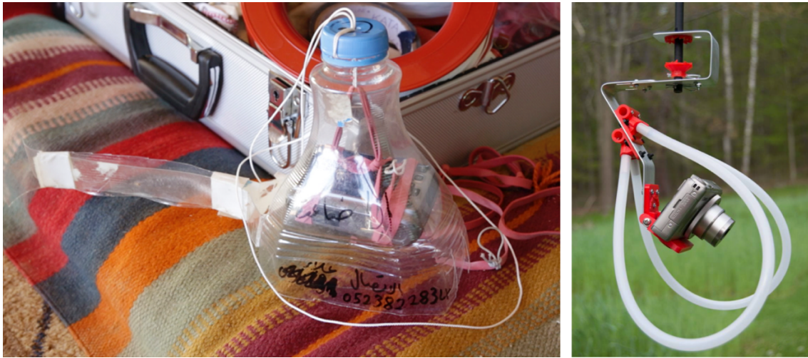
Figures 15a and b. (Left) The camera rig used in al-Araqib. The camera is held by a few rubber bands and pointed at 90° to the ground within a plastic bottle cut in two. (Image: Alina Schmuck & Jan Kiesswetter). (Right) A 3D-printed DIY camera rig also used in al-Araqib (Image: Chris Fastie). 22
